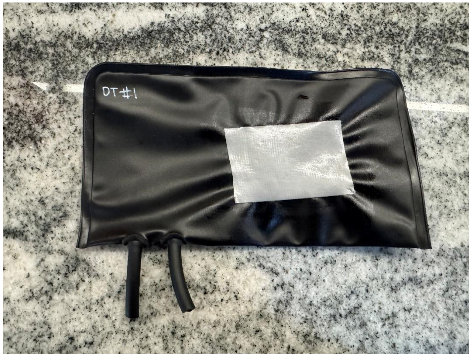
Figure 6A. Duct-tape repair outcome for Trial DT-1.
