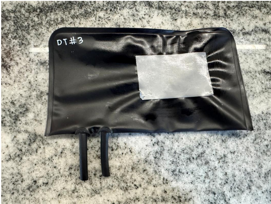
Figure 6C. Duct-tape repair outcome for Trial DT-3.
