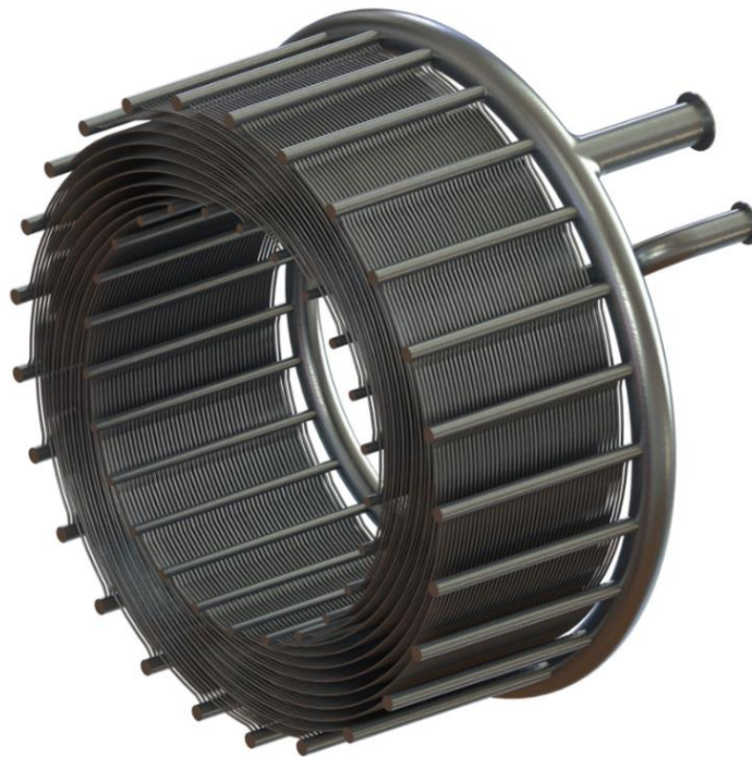
Figure-5. SABRE rocket engine design includes a precooler able to chill superheated air in a fraction of a second, allowing the engine to make use of oxygen from the atmosphere as it flies [Source: ESA]
