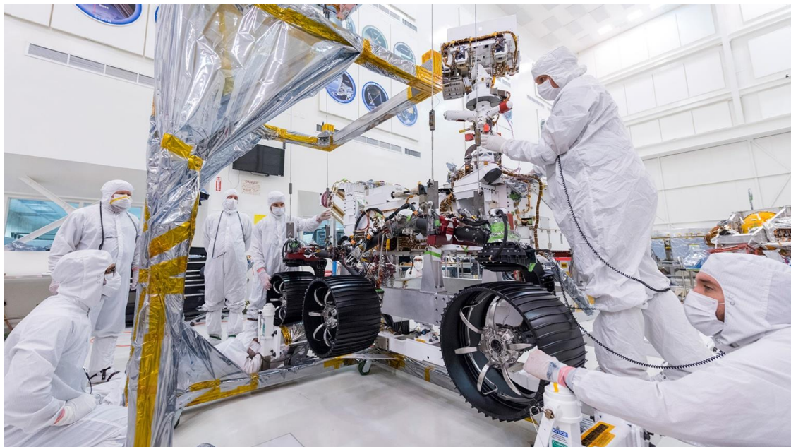
Figure 5: NASA Mars 2020 Perseverance rover illustrating the rocker-bogie suspension system, the reference mobility architecture adapted for contemporary planetary rovers including those planned for the lunar south pole. The passive-compliance linkage allows all six wheels to maintain ground contact independently on irregular terrain. From Mars 2020 Perseverance Rover: Rover Components [Photograph], by National Aeronautics and Space Administration / Jet Propulsion Laboratory – California Institute of Technology, 2021( https://mars.nasa.gov/mars2020/spacecraft/rover/ ). In the public domain.
