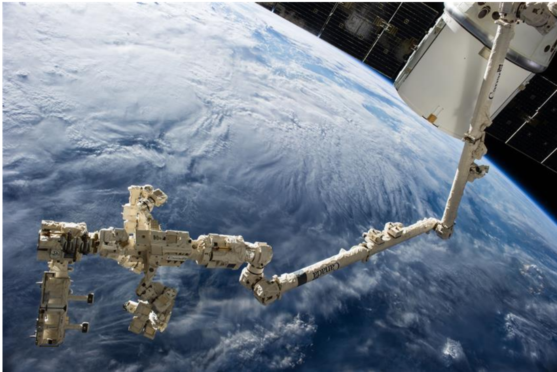
Figure 4: The Canadian Space Agency DEXTRE Special Purpose Dexterous Manipulator (SPDM) mounted on the International Space Station, demonstrating the concept of robot-executed orbital replacement unit (ORU) servicing that informs the design of autonomous maintenance systems for lunar surface infrastructure. From About the Special Purpose Dexterous Manipulator (DEXTRE)
