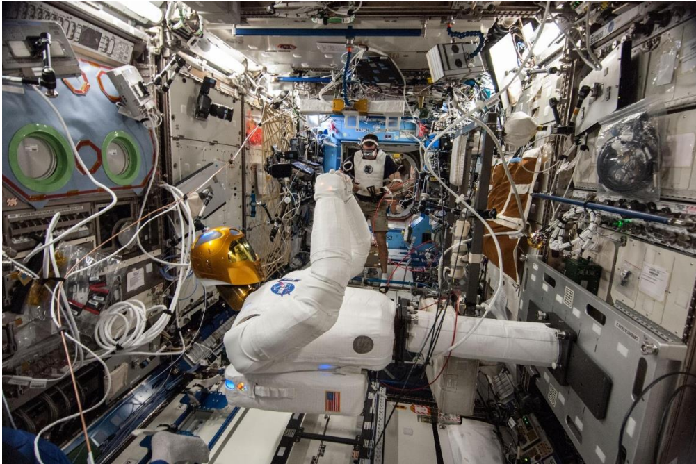
Figure 9: NASA Robonaut 2 (R2) humanoid robot on board the International Space Station, demonstrating dexterous two-armed manipulation tasks in the microgravity environment. R2 establishes the design precedent for humanoid robots capable of operating in human-designed workspaces, a capability directly applicable to future lunar surface maintenance operations. From About Robonaut 2 [Photograph], by National Aeronautics and Space Administration, Johnson Space Center, 2023 ( https://www.nasa.gov/robonaut2/ ). In the public domain.
