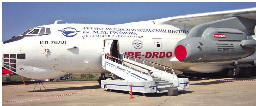
Figure 5. Kaveri mounted on a Russian IL-76 Flying Engine Test Bed. [30]
