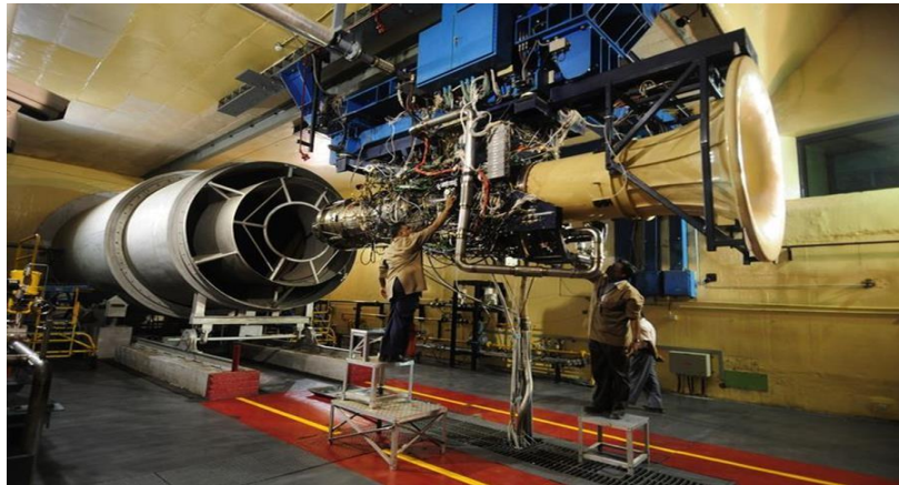
Figure 1. GTX-35VS Kaveri undergoing testing at GTRE in 2011. [31]
