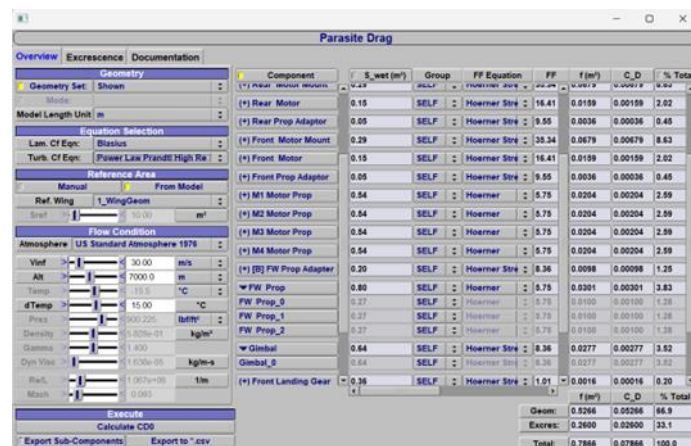
Figure 19 - Parasite Drag Estimation - OpenVSP
