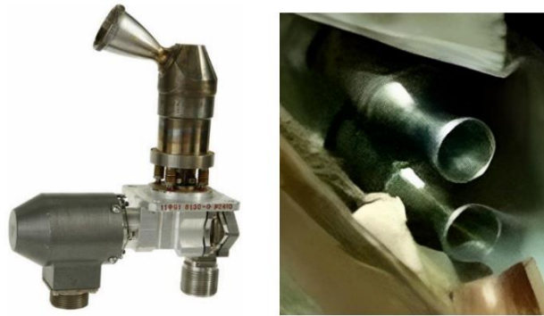
Figure-7. Soyuz HP Thruster [22, 23]
