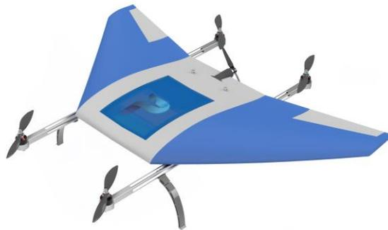
**Figure-10 3D CAD Model of Quadplane**
