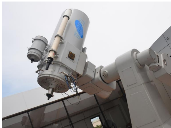
Figure-4 GOTO 45cm diameter Cassegrain reflection telescope at ACCIMT [10]
